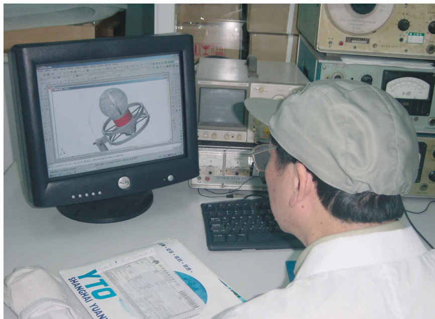
Fine-tuning the virtual plans for one of SE's mics in a computer-based CAD package.
