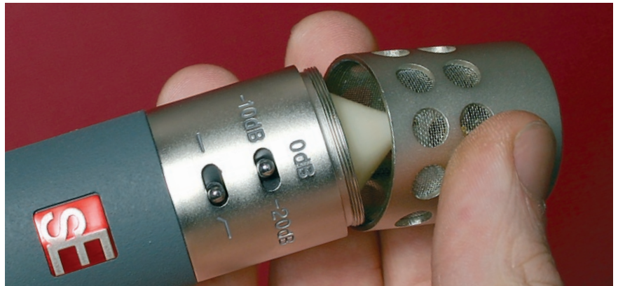
Like the earlier SE3, the cardioid capsule comes as standard, but on the SE4 it can be swapped for a hypercardioid or omni capsule, both of which can be purchased separately.
